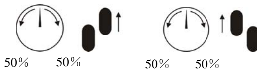
Fig. 6 rudder pedal directions to the turning direction of the pointer of the heading indicator
